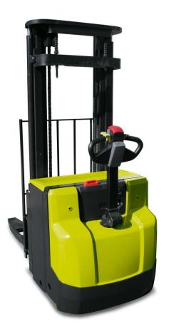
A real CLARK for warehousing and production applications: the electric high-lift truck SX 12/16 with load capacities of 1.2 and 1.6 tonnes and a maximum lifting height of 5.2 metres.
